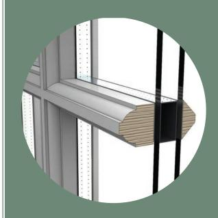
Simulated divided lights to match visually, original glazing bars. No thermal breaks around the perimeter of the glazing bars. Discreet double glazing with white back to back spacer bars, period mouldings and outer beads to match angled putty lines.
